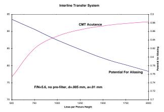
Figure 15. CMT Acutance and Potential for Aliasing as a function of lines per picture height for an Interline Transfer DSC.
