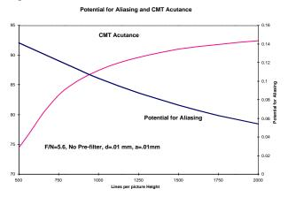
Figure 14. CMT Acutance and Potential for Aliasing for a monochrome Frame Transfer DSC as a function of the number of imaging lines per picture height.
