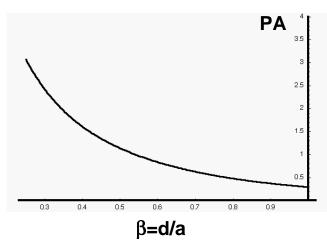
Figure 6. The Potential for Aliasing, PA, as a function of  $\beta = d/a$ . As the linear dimension, d, of the active area decreases for a fixed pitch, a, the Potential for Aliasing increases rapidly.
