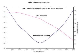
Figure 17. CMT Acutance and the Potential for Aliasing for a 2000 line, color, Frame Transfer DSC using a CFA plotted as a function of the image shift introduced by an optical pre-filter.
