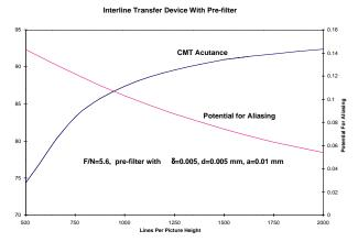
Figure 16. The CMT Acutance and Potential for Aliasing for an Interline Transfer device that has an optical pre-filter.
