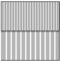
Figure 2. The top line pattern is sampled by a "pixel" that is three times the size of the pixels making it up. The resulting image on the bottom demonstrates an averaging over the larger pixel and the results of the three-fold sub-sampling.
