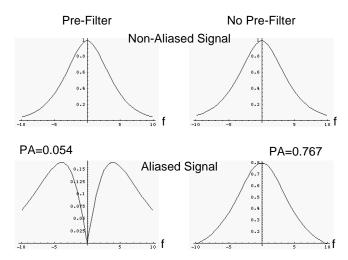
Figure 13. The above spectra are for the total system, including paper and laser printer and are based on the spectra shown in Figure 12. There is a dramatic reduction in the Potential for Aliasing when an optical pre-filter is introduced.
