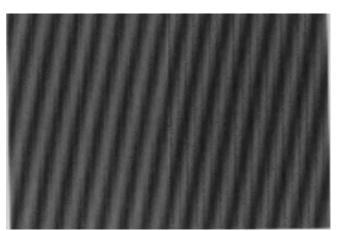
Figure 4. This is the aliased image of a test chart taken with a consumer Digital Still Camera. The test chart has a frequency of 80 line pairs per target width. As can be seen from the above image, there are approximately 15 line pairs, showing the strong aliasing that has taken place.
