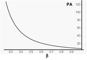
Figure 10. The Potential for Aliasing for the red or blue sampling structure of the Bayer CFA. Note that the Potential for Aliasing is twice that of the green sampling structure and four times that of a monochrome sensor; see Figure 9.
